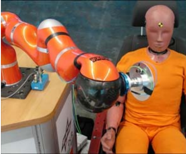
Standardized crash tests for the evaluation of “Safety in physical Human-Robot Interaction”
