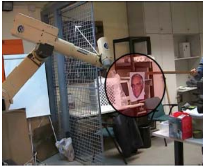
Figure 4. Face detection and avoidance in an industry-like robotic cell
