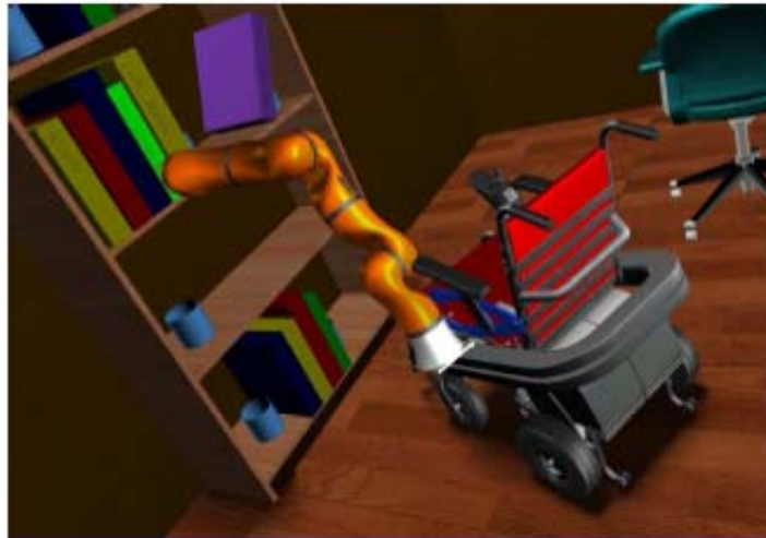
Figure 5. Virtual environment for assistive robotics evaluations
